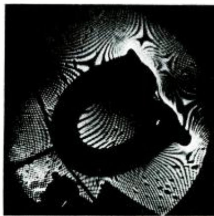
Fig. 4—Pattern of a horseshoe magnet.
